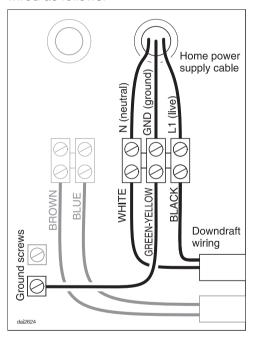
Black wire: . . . . . connect to L1 (live) White wire: . . . . connect to N (neutral) Green-yellow wire: . . . connect to GND . . . . . . . . . . . . . . . . . . (ground)
